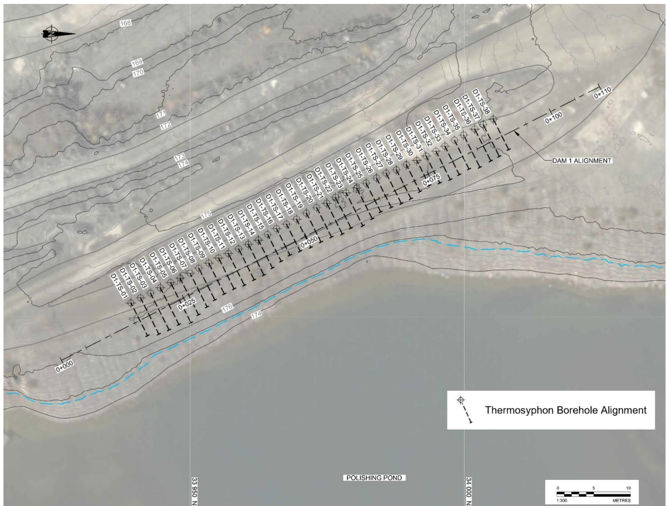
Figure 16: Dam 1 Thermosyphons Alignment
