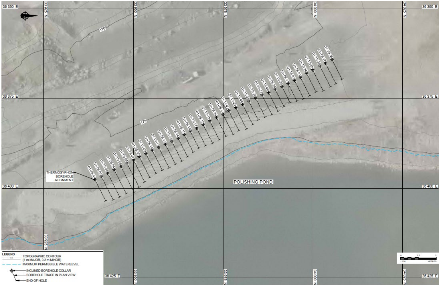
Figure 16: Dam 1 Thermosyphons Alignment
