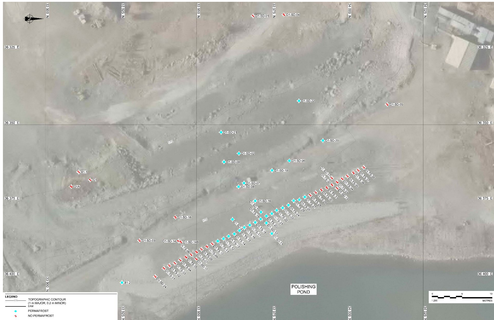
Figure B-2: Dam 1 Overview – Permafrost Locations (Geocon 1975, 1983; Golder 2019b, 2021a)
